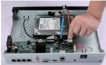
4. Connect one end of the data cable to the motherboard of NVR.
