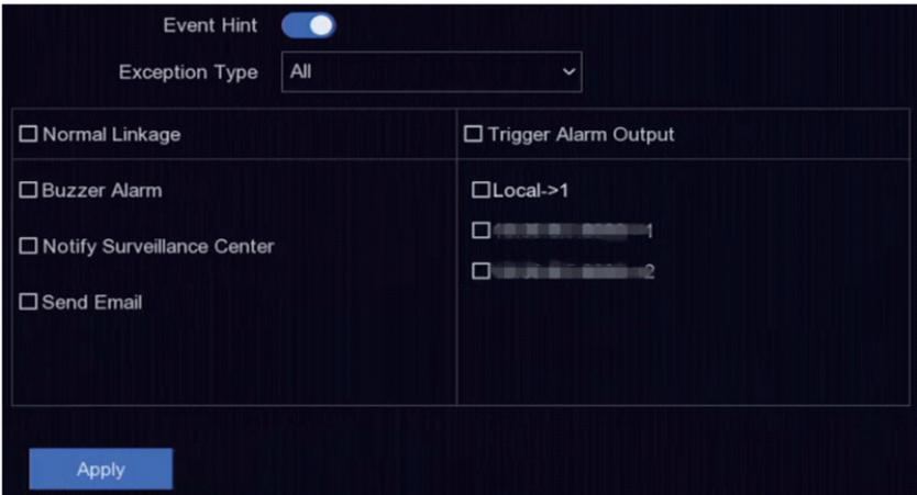
The screenshot shows the 'Exception' configuration page. At the top, there is a toggle for 'Event Hint' which is turned on. Below it is a dropdown menu for 'Exception Type' set to 'All'. The main area is divided into two columns of checkboxes. The left column contains: 'Normal Linkage', 'Buzzer Alarm', 'Notify Surveillance Center', and 'Send Email'. The right column contains: 'Trigger Alarm Output', 'Local->1', and two blurred options. At the bottom left, there is a blue 'Apply' button.
