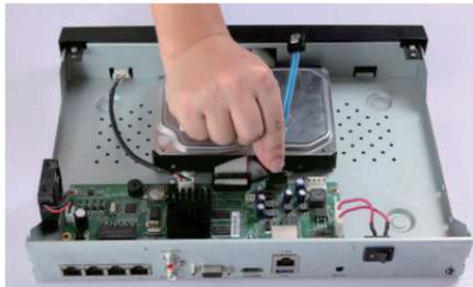
5. Connect the data cable and the power cable to the HDD.
