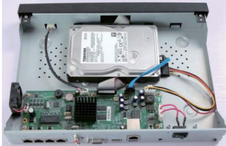
6. Place the HDD on the bottom of the device and then fasten the screws on the bottom to fix the HDD.
