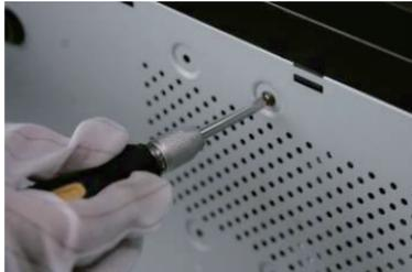
7. Re-install the cover of the NVR and fasten screws.
